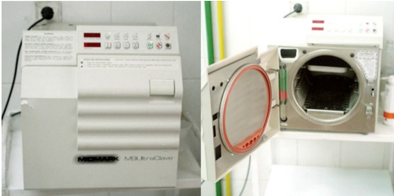
Fig. 2. Steam Autoclave use steam under pressure with/without vacuum the use of vacuum is more efficient. Instruments must be wrapped or packed. Instruments are left inside for 15-20 minutes at 135 °C.
